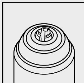
13 mm solid metal drill chuck for use with commercially available shank, such as cylinder and hexagon shank.
