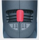
Clockwise/anti-clockwise switch on the top of the housing ensures maximum torque in both rotation directions via optimum positioning of the carbon brushes and extends the service life of the carbons.
